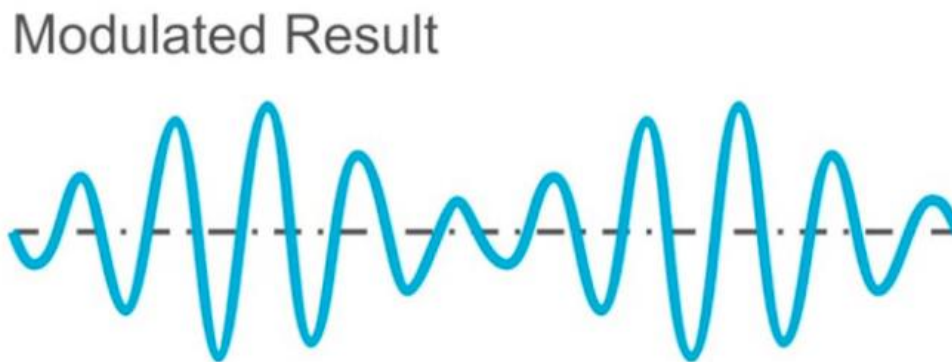
Figure 20 Resulting Amplitude Modulated Signal reprinted with remission from: www.taitradioacademy.com
